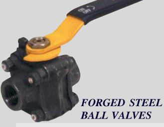
Forged Steel ASTM A 105 Ball Valve, Three Piece Design, Regular Port, BSPT/NPT Socketweld, Butt-weld end, ANSI 800 #.
